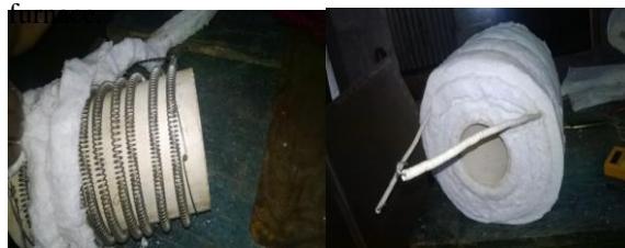
Fig 15 Wrapping of ceramic blanket around the coil and pot
