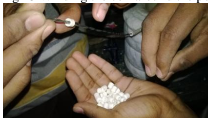
Fig 14 Covering the coil with ceramic beads
