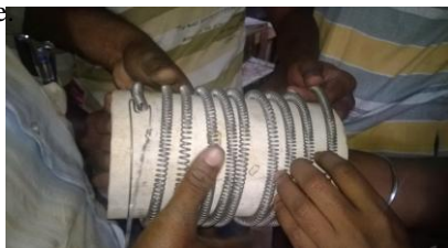
Fig 13 Winding the coil around the pot
