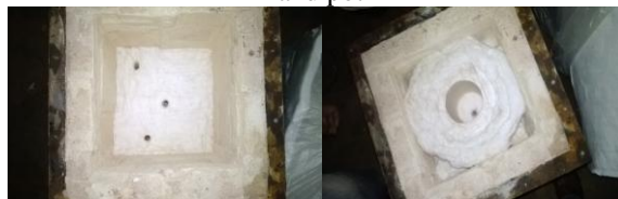
Fig 16 Drilling holes through the base and inserting the pot in the furnace
