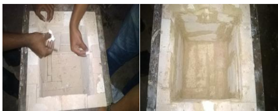
Fig 12 Packing ceramic blanket pieces and applying the ceramic paste
